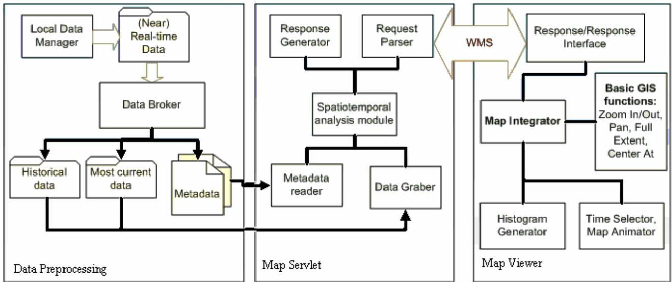
Figure 2. Framework design: *data preprocessing* modules provide geospatial data and metadata so that interoperable communications can be performed between *map servlet* and *map viewer*.
