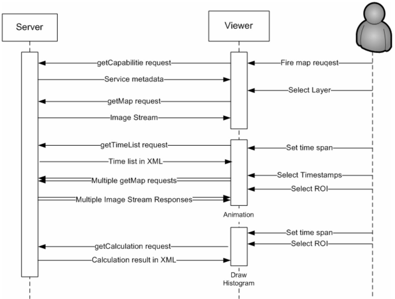
Figure 4. Client server communication for the scenarios of real-time WMS, map animation, and spatiotemporal analysis.
