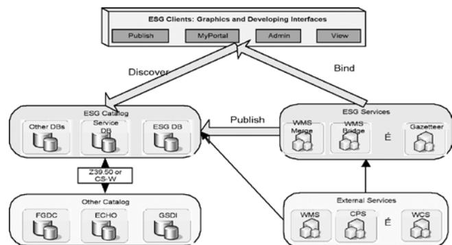
Figure 3. The ESG logic architecture
