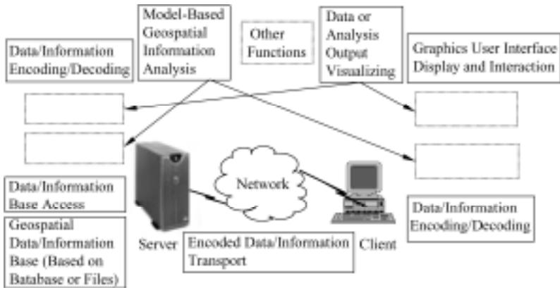
**Figure 16.4** A flexible distributed GIS framework: the server side hosts data, provides data access interface; the client side displays the visualized data/output and interacts with users; data/information transmitted through the network will be decoded/encoded at both client and server side; model-based analysis, data visualizing, and other functions can be hosted at either server side or client side
