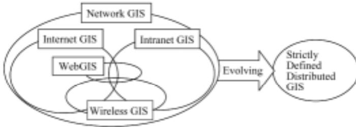
**Figure 16.5** Network GIS taxonomy: different terms of network GIS refer to different implementations of distributed GIS: Network GIS is implemented in a network, which includes all kinds of GIS built on computer network; Intranet GIS is implemented in the Intranet. Internet GIS is implemented within an Internet. WebGIS is implemented inside a web browser. Distributed GIS is a future Network GIS with transparent characteristics that require more research and development
