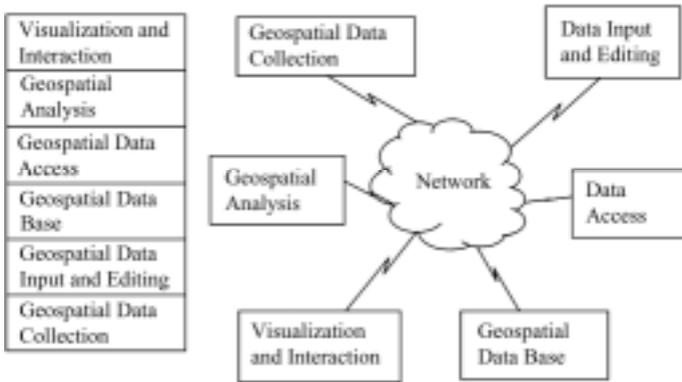
**Figure 16.3** A traditional monolithic GIS (left) and a networked GIS (right) with different GIS functions distributed in a computer network. These functions can be allocated on two or more than two computers
