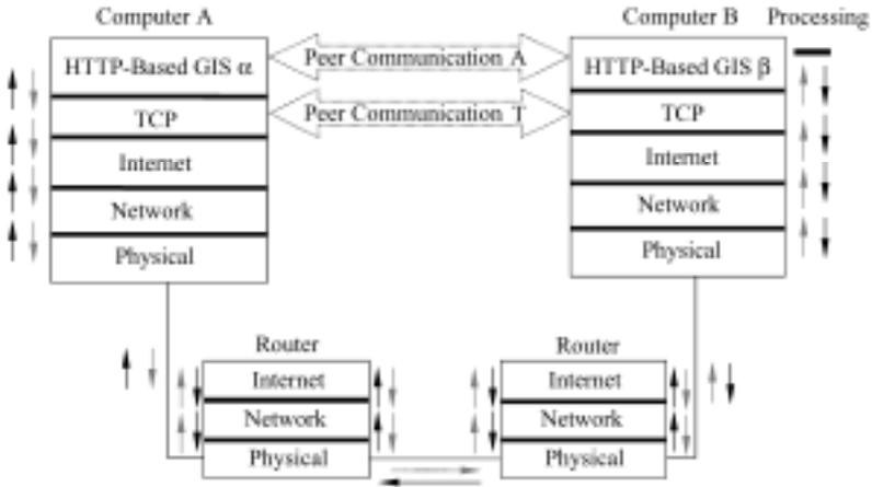
**Figure 16.2** The communication procedure between two GISs in the Internet: The gray arrow shows the information flow of request from  $\alpha$  to  $\beta$ , and the black arrow shows the response from  $\beta$  to  $\alpha$
